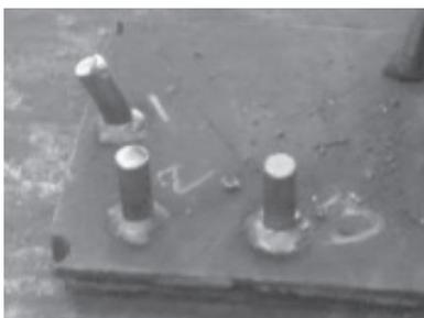
*Fig 1: Pin bent after hammering*
