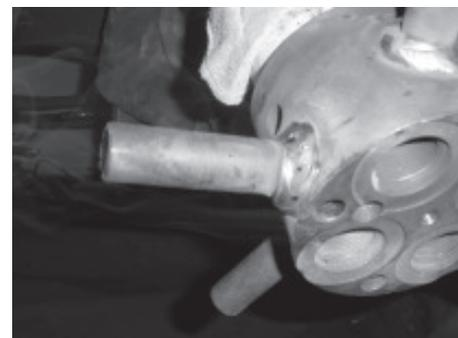
*Fig 2: Pin welded to shaft*
