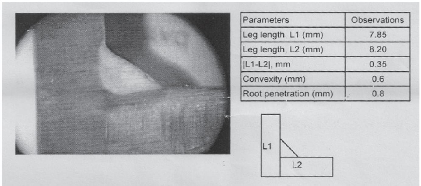
Fig 4: Cross-section of the weld
